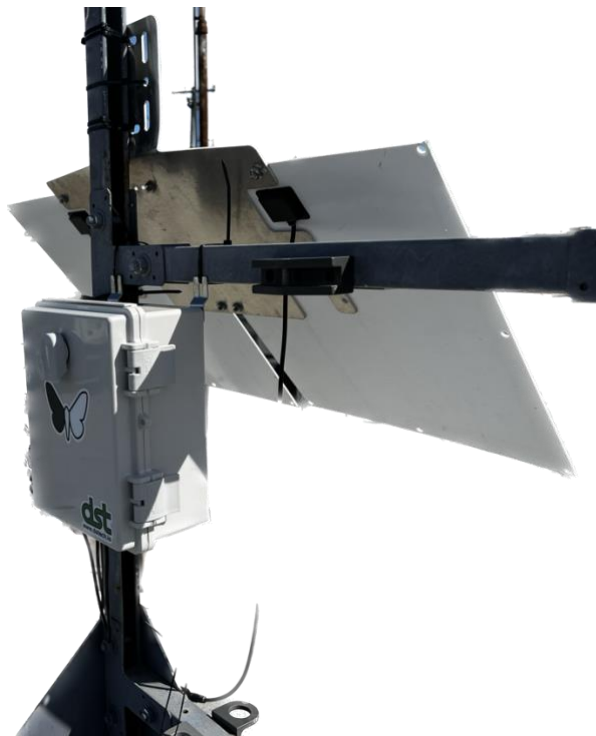
Figure 12. Mounted enclosure showcasing orientation with the inlet/outlet facing the ground.
